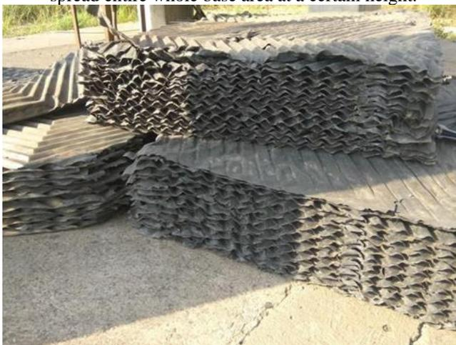
**Fig.3 PVC Fill material**
