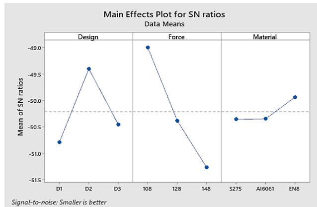
Figure 10: Main effects of plot for SN ratios
