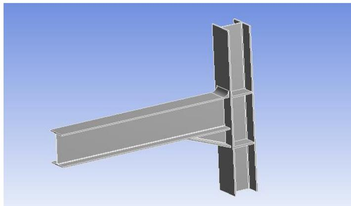
Figure 4: Design 2 showing curve joint perpendicularly
