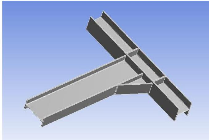
Figure 3: Design 1 showing direct joint of beams perpendicularly
