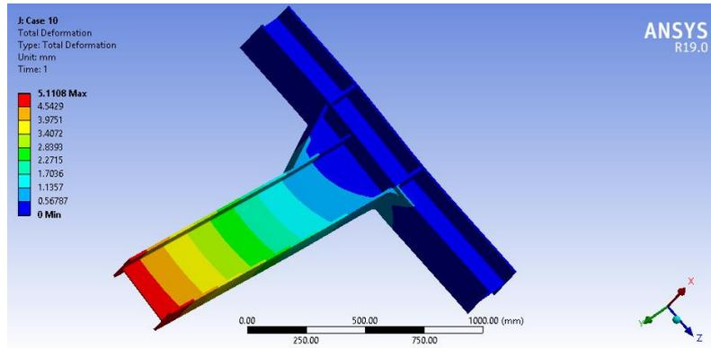
Figure 12: Total deformation
